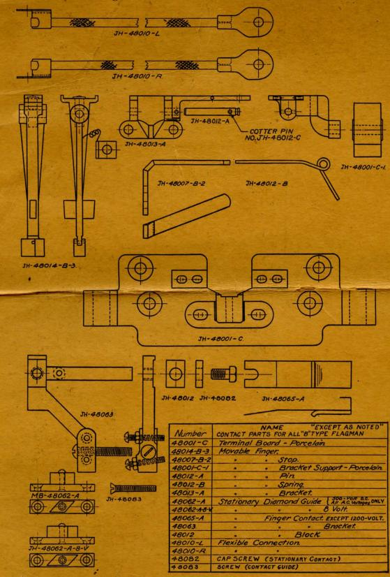
Due to the increased number of parts in the three position locking mechanism a more careful inspection of wearing surfaces, catches and springs should be given.
