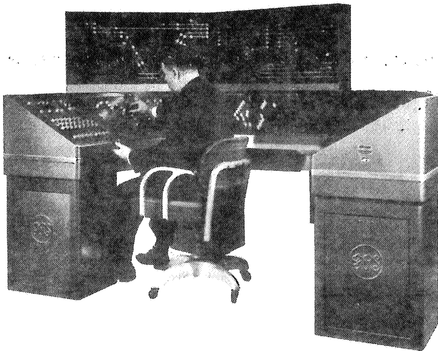
Fig. 14. Console Route Type (NX) Control Machine with Separate Track Diagram.
