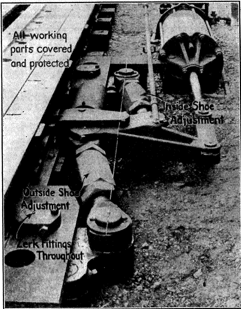
Fig. 24. Linkage of Model 28 Retarder in Open Position.
