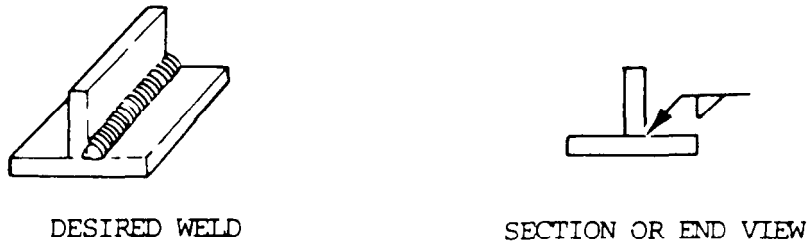
Figure 3-9. Arrow side fillet welding symbol.
