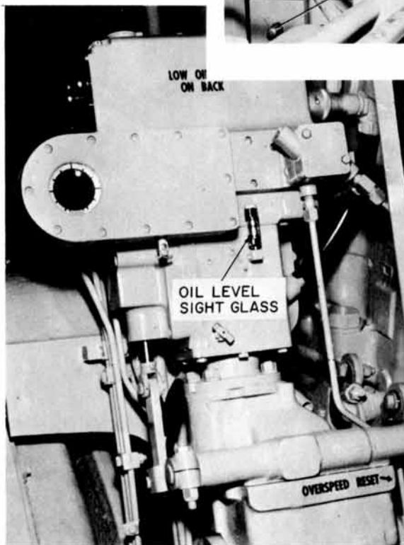
Fig. 13. Engine control governor and low-oil and low-water resets
