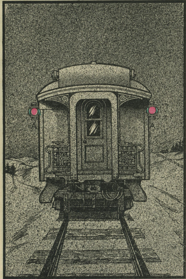
Fig. 13. REAR OF A TRAIN AT NIGHT WHILE RUNNING. Lights at A A, as Markers, showing GREEN toward the engine, and side, and RED to the rear.
