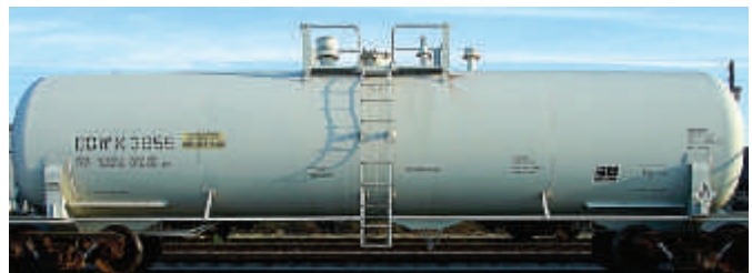
General Service (Low Pressure) Tank Car: Note the exposed fittings at the top and underneath the car
