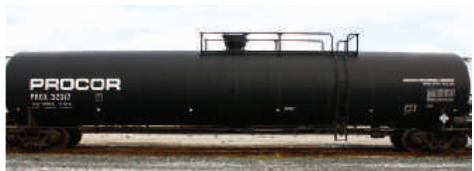
High Pressure Tank Car: Note the single protective housing at the top of the car and no fittings underneath the car
