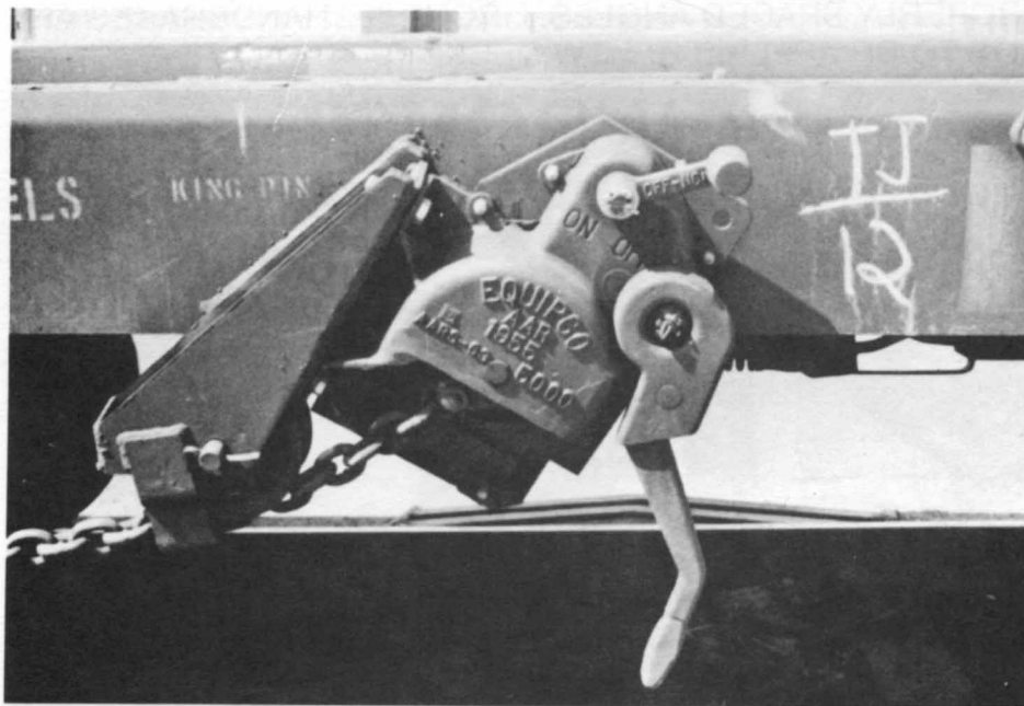
THIS TYPE HANDBRAKE, GROUP "F" ARE NOT TO BE APPLIED ON TTAX/TTCX TYPE CARS. THESE TYPES CANNOT BE PROPERLY OPERATED FROM SIDE OF CAR. (SEE NOTE "B" BELOW).
