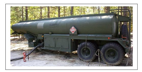
Figure 3-3. M969 5,000-gallon semitrailer.
