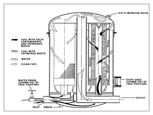
Figures 1-1. Typical flow through a filter/separator
