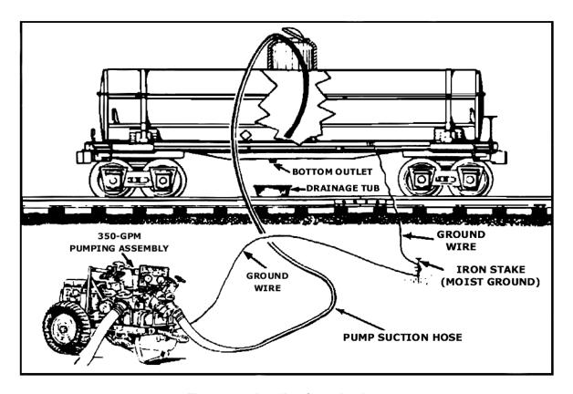
Figure 3-8. Loading from the dome.
