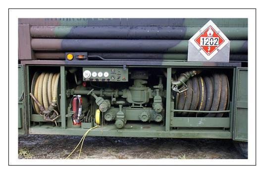
Figures 3-2. M131A5C 5,000-gallon semitrailer (cabinet doors open).
