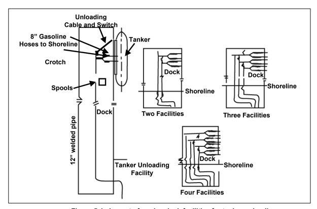
Figure 5-1. Layout of marine dock facilities for tanker unloading.
