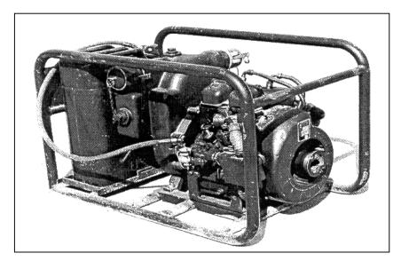
Figures 2-2. The 100-GPM pumping assembly.
