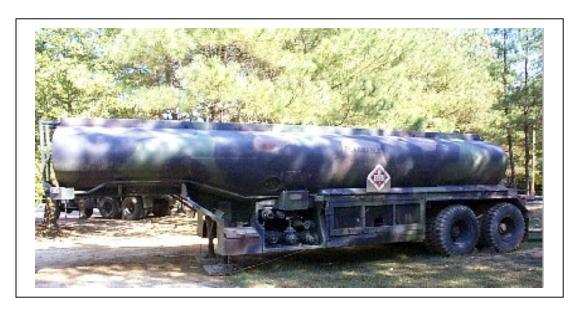
Figure 3-4. M970 5,000 gallon semitrailer
