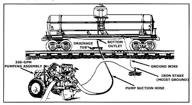
Figure 3-7. Loading from the bottom.
