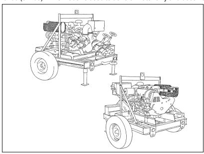
Figures 2-3. The 350-GPM pumping assembly.
