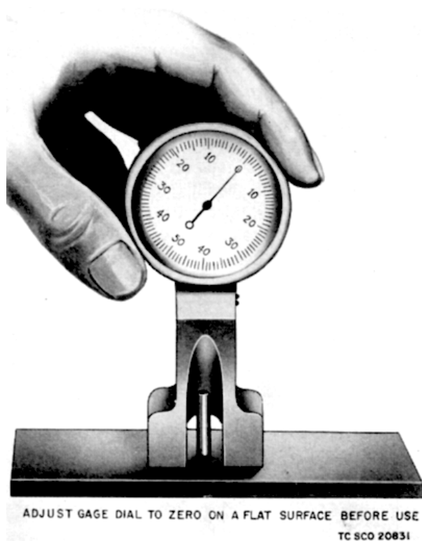
Figure -23. Micrometer dial gage for adjusting magnet valve.
