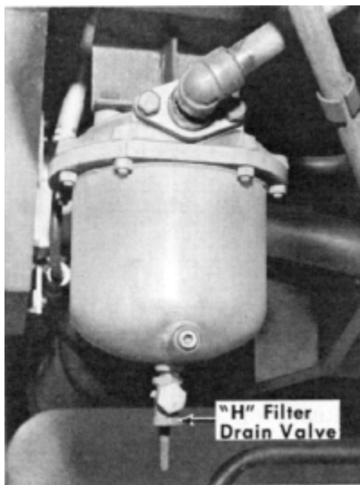
Fig. 4-13 - "H" Type Filter
