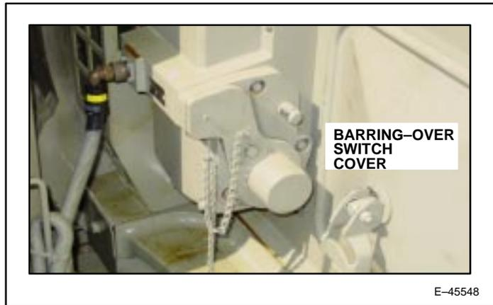
Figure 30. Engine Barring-Over Switch.
