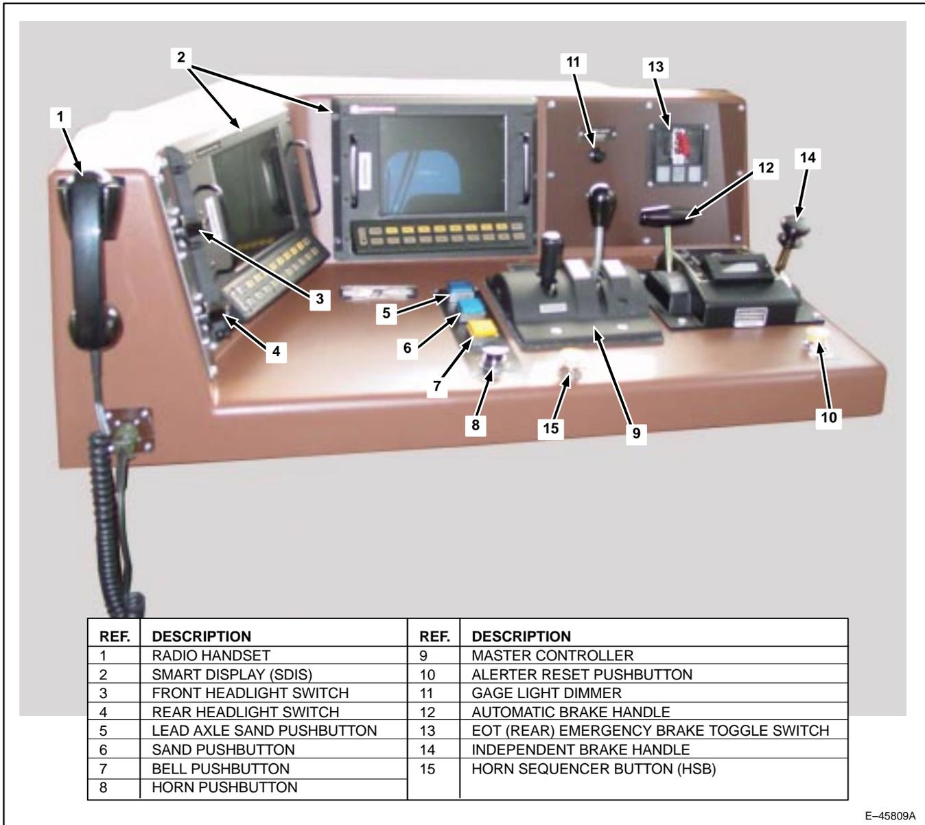
Figure 5. Operator Control Console, Top.
