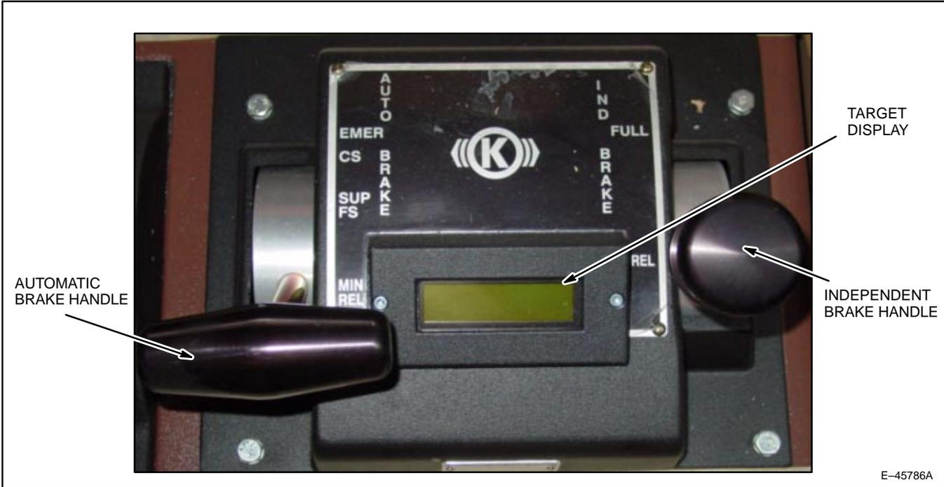
Figure 12. Electronic Air Brake Controller (EBV).
