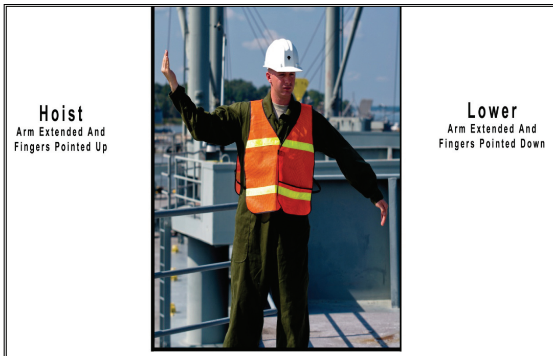
Figure 3-10. Signals Used in Winch Operations (Two Winches)
