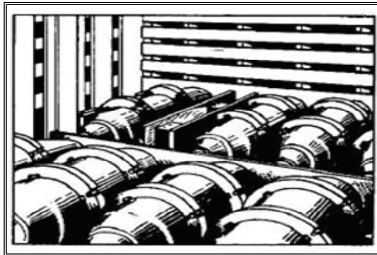
Figure 9-11. Dunnage Used to Separate Bombs
