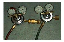
With the pressure in a full Acetylene cylinder at 250 psig and a full Oxygen cylinder at 2200 psig, a way is needed to lower these cylinder pressures to desired working pressures for use in the torch. This is accomplished by using an adjustable pressure reducing regulator. The regulator will also maintain a steady working pressure as the cylinder pressure drops from use.
