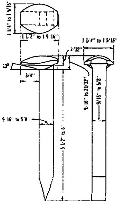
Figure 3.9. Details of Cut Spike.
