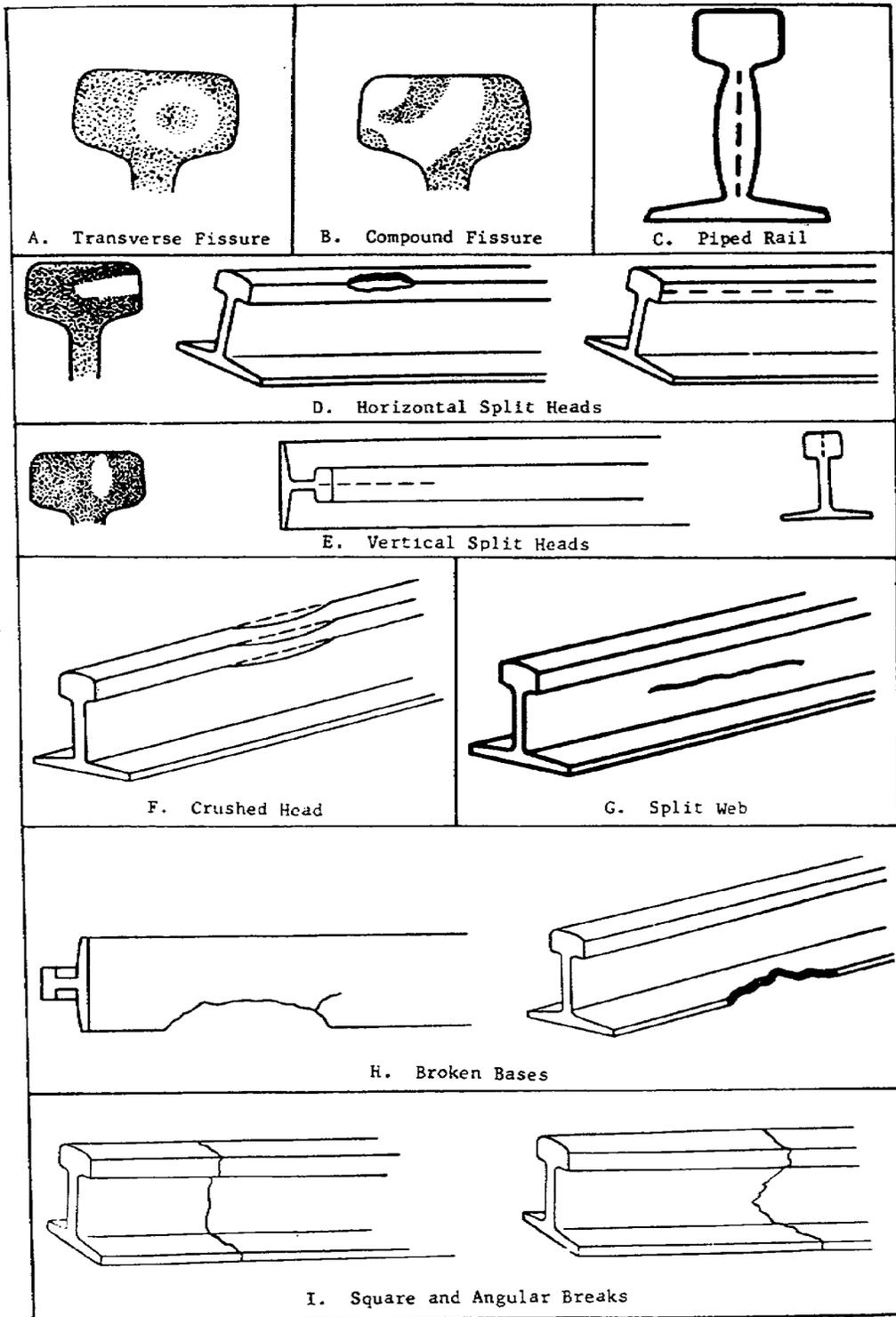
Figure 3.2. Rail Defects.
