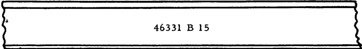
This means that the rail came from heat No. 46331 and was the second rail rolled from the 15th ingot poured. If CC appeared here, it would indicate that the controlled cooling process was used. Similarly, CH stands for controlled cooling and end hardened. End hardening is a special process that reduces the effect of excess wear at the joints (par. 3.29).
