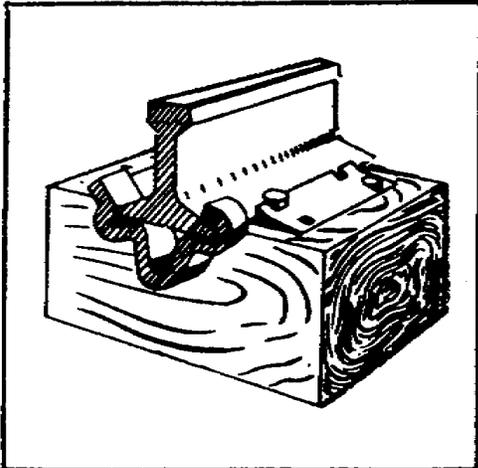
Figure 3.14. Typical Rail Anchor.
