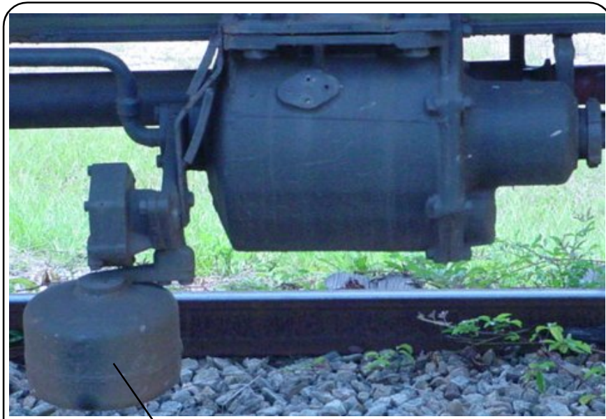
Modulating Valve Applied to Brake Cylinder
