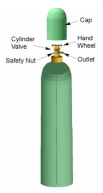
The oxygen volume in a cylinder is directly proportional to its pressure. In other words, if the original pressure of a full oxygen cylinder drops by 10% during welding, it means 1/10th of the cylinder contents have been consumed.
