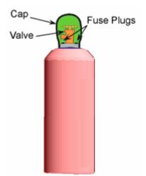
Acetylene is extremely **unstable** in its pure form at pressure above 15 PSI. This instability places special requirements on the storage of acetylene. Acetylene cylinders are packed with porous material (balsa wood, charcoal, corn pith, or portland cement) that is saturated with acetone to allow the safe storage of acetylene. These porous filler materials aid in the prevention of high-pressure gas pockets forming in the cylinder.
