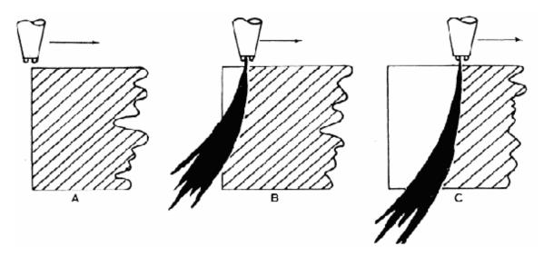
Progress of a cut in thick steel
