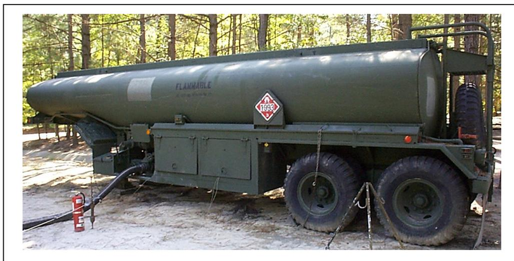
**Figure 3-3. M969 5,000-gallon semitrailer.**
