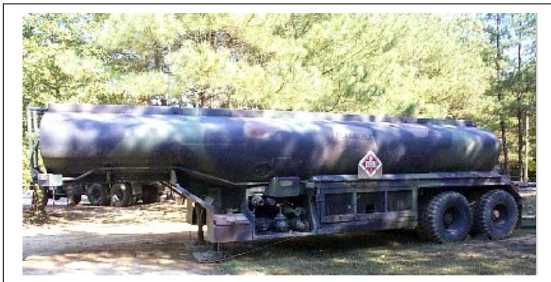
**Figure 3-4. M970 5,000 gallon semitrailer**
