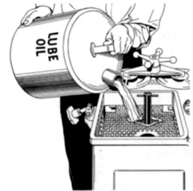
Adding Oil To Engine Fig. 4-5
