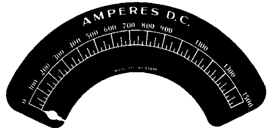
Load Indicating Meter Fig. 2-8
