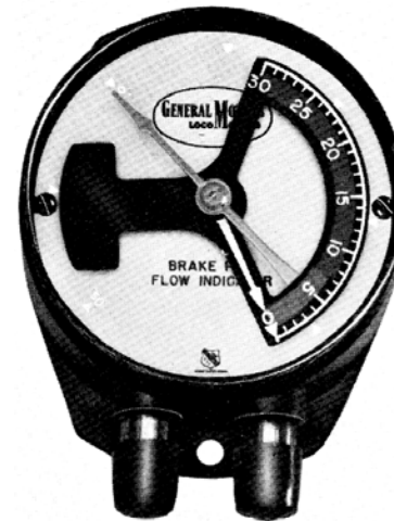
Uncharged Train Or Dead Brake Pipe Fig. 2-19
