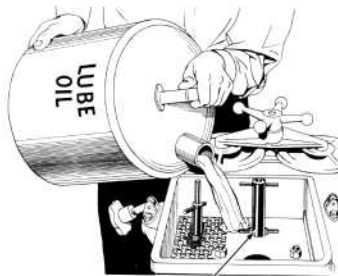
Strainer Drain Valve Open ONLY if draining the engine oil pan
