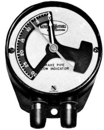
Brake Pipe Flow Indicator Fig. 3-6
