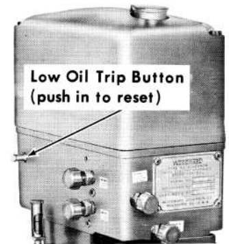
Governor Low Oil Pressure Device Fig. 4-7
