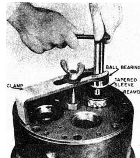
Cleaning Valve Guide Fig. 2-20
